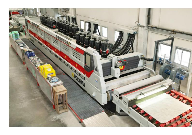
EN Pedrini presents the innovative GALAXY MX-T2 and GALAXY MX-T3, a new version of a marble slab polishing machine available in the models with two or three moving beams and designed to perfect the polishing process.
