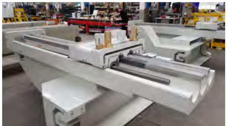
*The bridge is assembled onto two sliders that slide along the columns with the interposition of anti-friction slides. A prismatic guides system that has been machined onto the columns structure, reacts to stress coming from any direction and guarantee perfectly straight bridge vertical stroke.*
