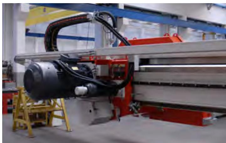
The **disc-holder trolley** houses a set of important components:
